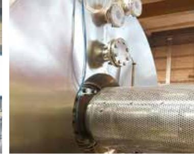
Spacer for Shaft Seal Removal
