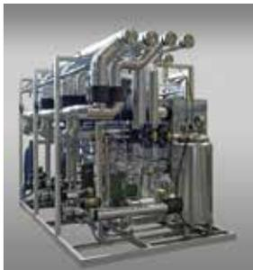
The heating and cooling skids are used for heating or cooling the jackets of agitated vacuum dryers, agitated Nutsche filters and filter dryers with heat transfer fluid 15 - 300 kW heat transfer capacity 4 –150 m<sup>3</sup>/h flow rate.
