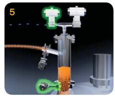
The powder outlet valve opens and pressurized nitrogen helps discharge the solids into the receiving vessel. The nitrogen valve remains open, preventing oxygenated/solvent laden air from entering the Powder Pump body.
