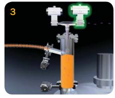
When the pre-determined transfer time has elapsed, the powder inlet valve closes. A brief delay allows residual air to be evacuated; then the vacuum isolation valve closes.
