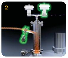
After a pre-set time, the powder inlet valve opens and solids are drawn into the body. Entrained gas is evacuated through the internal dust filter, and the solids are retained inside the body.
