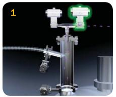
With the vacuum source in operation, the vacuum isolation valve opens to remove oxygenated or solvent laden air from the Powder Pump body.
