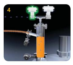
Next, the nitrogen isolation valve opens, creating a back-pulse of nitrogen to clean the dust filter, as well as relieve the vacuum and inert the Powder Pump body.
