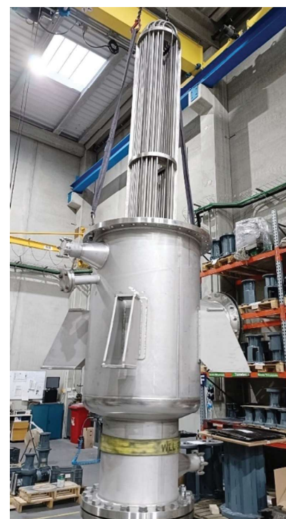
Shell and Internal Condenser
