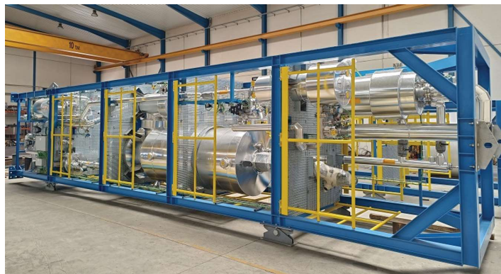
5m2 horizontal preassembly short path installation at our workshop
